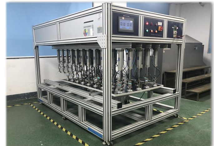
±1000Pa + 1000cycles Dynamic Mechanical Load Test
