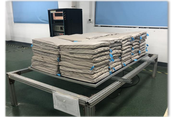
+5400/-2400 Pa Static Mechanical Load Test
